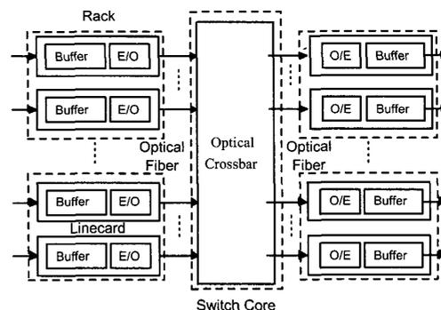
Fig. 1. Schematic view of a multi-rack hybrid packet switch.
