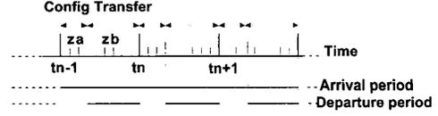
Fig. 5. Execution time line of single schedule+hold algorithm.
